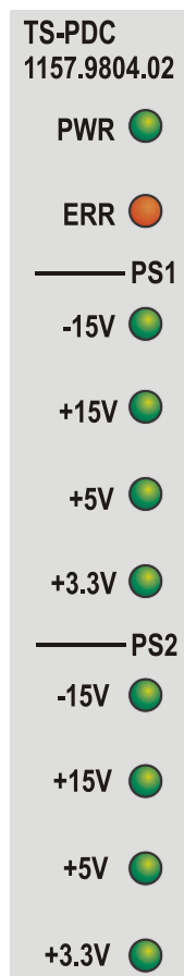
Figure 4-4: LEDs on the R&S TS-PDC module from Version 2.0
